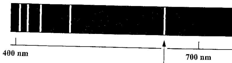
Figure 1. Wavelengths of the most prominent lines in the visible region of the atomic hydrogen spectrum
